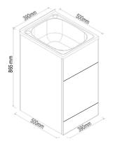
Size: 385x495x865 mm Thickness: 0.8 mm Material: MDF Capacity: 27 litre
